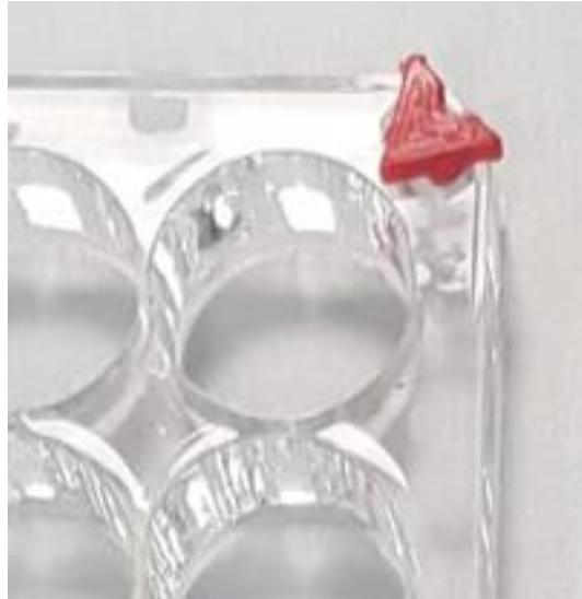
This very small arrow is inserted into the laser cutter plexiglass racks. We use it in order to remember the operator that A1 of the 1st rack is a fake sample (always negative). It's the only component which should be printed with a different color with respect to the t-gläse (which is white).
