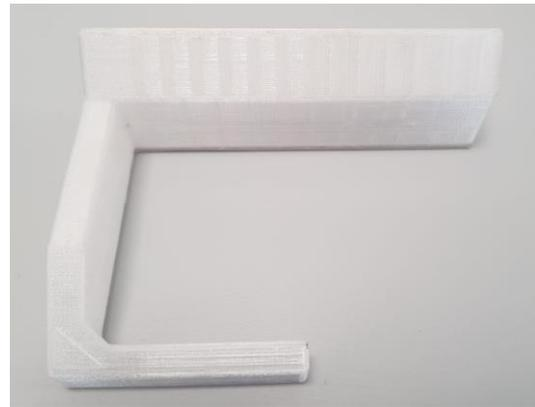
This device is basically a “filling mask”. It’s used outside the robot in order to prepare the 12 deep-well plate with all the different reagents. The empty deep-well plate is inserted from right and the bottom left corner has the same chamfer of the plate in order to avoid possible misalignments. If correctly positioned, the vertical bars should align with the cavities of the plate. Sticky labels may be placed above the bars to facilitate the identification of the position of the reagents.
