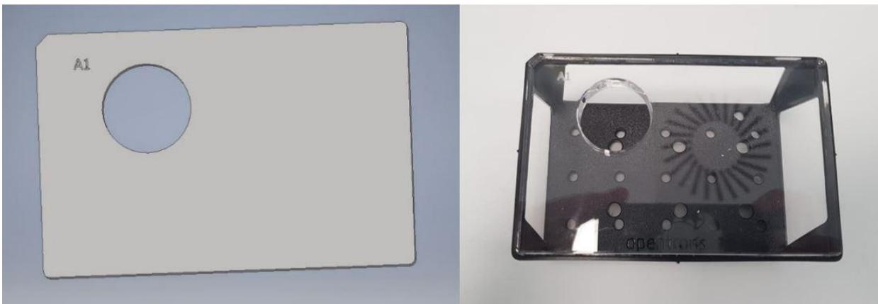
The six-position rack top is designed for specific application due to the working process. Only one hole exists on the top rack (due to the reason that only A1 position hole will be used in this station ) to avoid wrong placement.
