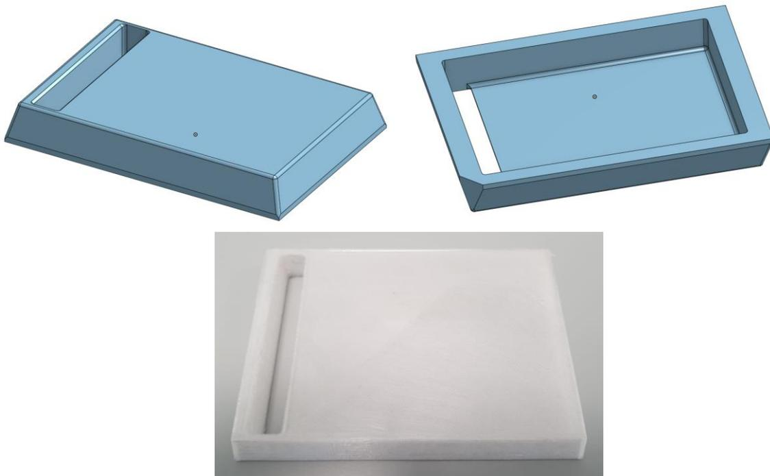
This mask is a replacement for the black plastic mask which Opentrons uses above the aluminum block. The original purpose is to avoid heat exchange and keep the plate cold for as long as possible. Since many holes are not used (in fact only the first row is filled), we improved the original piece by covering all the unused holes, so that we can avoid wrong positioning and keep the plate cold for a longer time.
