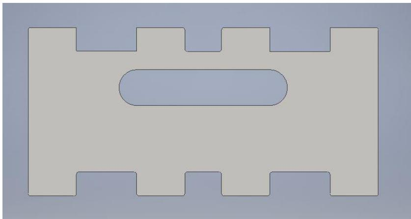
To make the rack more stable, we add two side-parts which allow operators to carry and move the rack easily by putting fingers inside the big hole in the middle.
