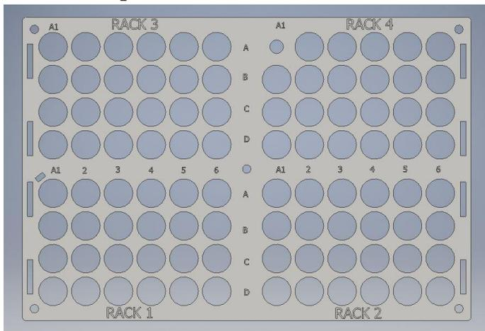
The picture above is the 96-top. The small rectangular hole near A1 position hole in RACK 1 is for inserting the indicator arrow (see Section 1.5) in order to remind operators the difference. As for RACK 4, the A1
