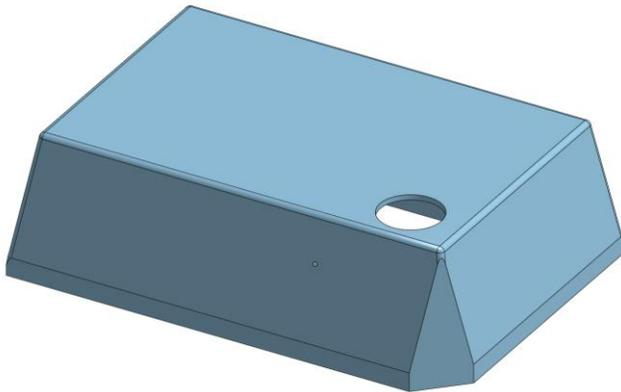
This mask prevents wrong positioning of the tube in station C. Moreover, it avoids the plate to heat up since it covers the aluminum block almost entirely. Notice that we have a chamfer to define the right orientation.
