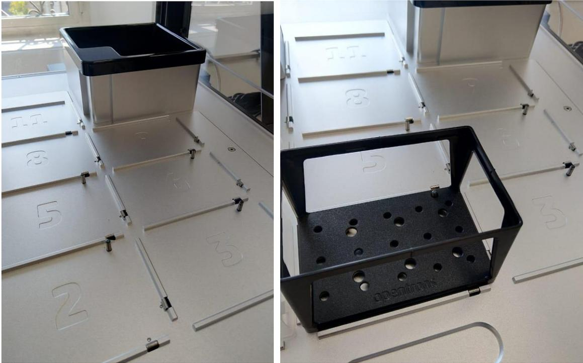
First, we drilled holes in the deck of the Opentrons robot with the help of the drilling guides (see Section 1.2). Then we tapped the holes, created the internal threads to screw the pins (i.e. stainless steel bars with an external thread) onto the deck of the Opentrons robot. By adding simple holes on the base of the racks, we created asymmetric features that help operators place the rack in the correct orientation.
