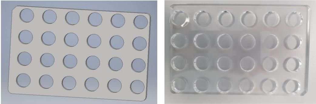
The top weight part is designed to avoid the pipette tip being stuck (due to the vacuum created in between) inside 10mm tubes by adding weight from the top of tubes. The dimension of the holes is smaller than the one of upper edge of the tubes which ensures the area to apply force caused by weight, in the meanwhile it is also big enough to let the operators place top-weight part easily above the rack top.
